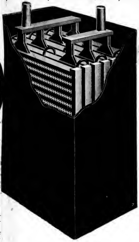
Fig. 1. View of Battery Element.
